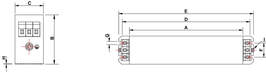
**Dimensions (unit: mm)** Tolerances according to ISO 2768-m / EN 22768-m
